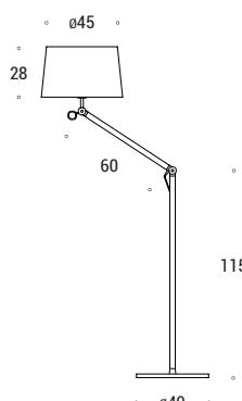
Floor lamp with adjustable and extendible frame. Conical fabric shade. Transparent power cable with on/off switch.
