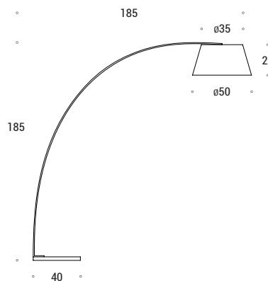
Floor lamp with arc stem and fabric diffuser. Marble base in the same colour as the shade. For lamp with E27 fitting, max. 40W. ON/OFF foot switch on the power cord.
