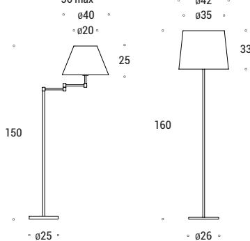
Floor lamp for LED E27 light bulb for ambient lighting. Steel structure and fabric shade. For ambient lighting and diffuse light effect.
