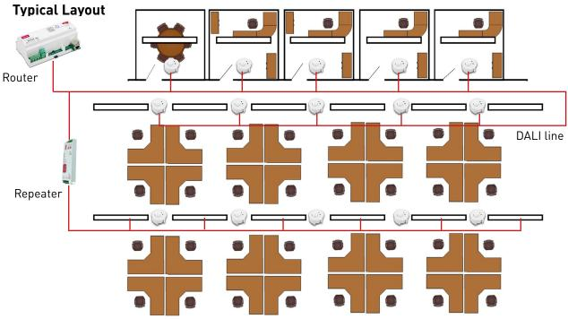
Note: This solution does not provide additional DALI addresses. The DALI limit of 64 addresses still applies.
