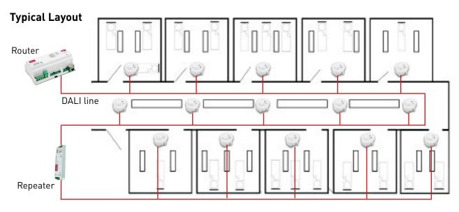
Note: This solution does not provide additional DALI addresses. The DALI limit of 64 addresses still applies.
