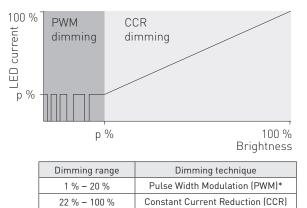
PWM dimming frequency 1 kHz
