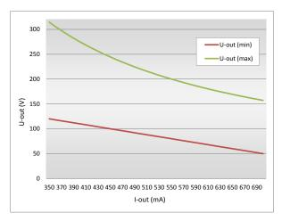
$U_{out}(max) = 110 \text{ W} / I_{out}$  $U_{out}(min) = (-0.2 \text{ V/mA}) \times I_{out} + 190 \text{ V}$
