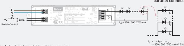
Note: Not suitable for load side switching operation.
