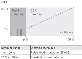
\* PWM dimming frequency 800 Hz
